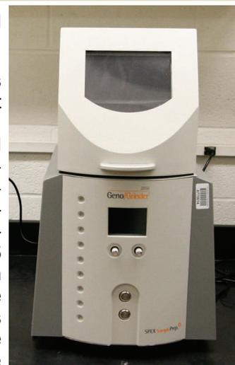
**The Gino/Grinder** has the capacity of homogenizing 84 samples at once and
